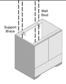
Drill holes in back support brace at wall stud locations. Fasten vanity to wall using fasteners of your choice through the support brace into wall studs.
