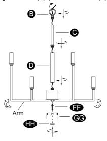
3. Determine the height that you would like to hang your fixture. Trim the cord and chain. Allow 10" of extra wiring for the electrical box connections.
