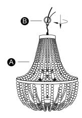
2. Determine the height that you would like to hang your fixture. Trim the cord and chain. Allow 10" of extra wiring for the electrical box connections.
