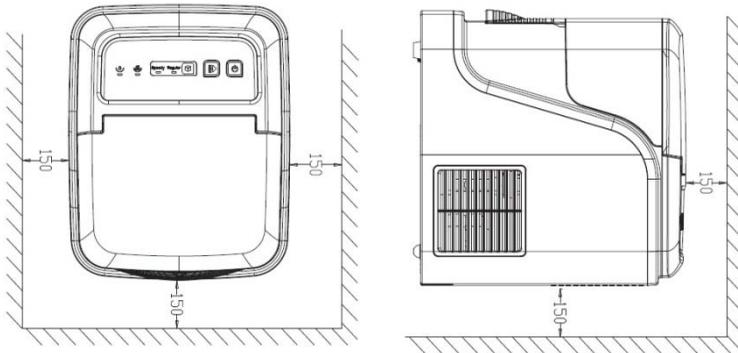
The machine should be upright to place on the horizontal plane. To ensure the machine ventilate normally, it is important to set 150mm room on top, sides and back. Do not place the machine next to the roast oven, radiate or other heat objects.
